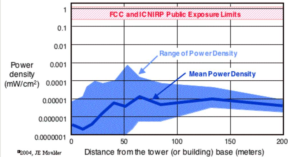
The relationship between the RF power density and distance from the base of the tower or building on which the mobile phone base antenna was located.
