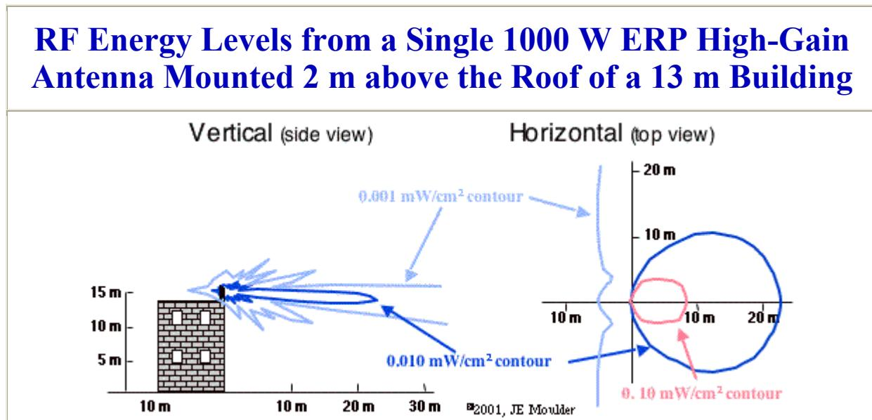
Keep in mind that mobile phone base station that use high-high-gain sectored antennas will usually use 3 (or occasionally 4) of these transmission antennas, all pointing in different directions.
